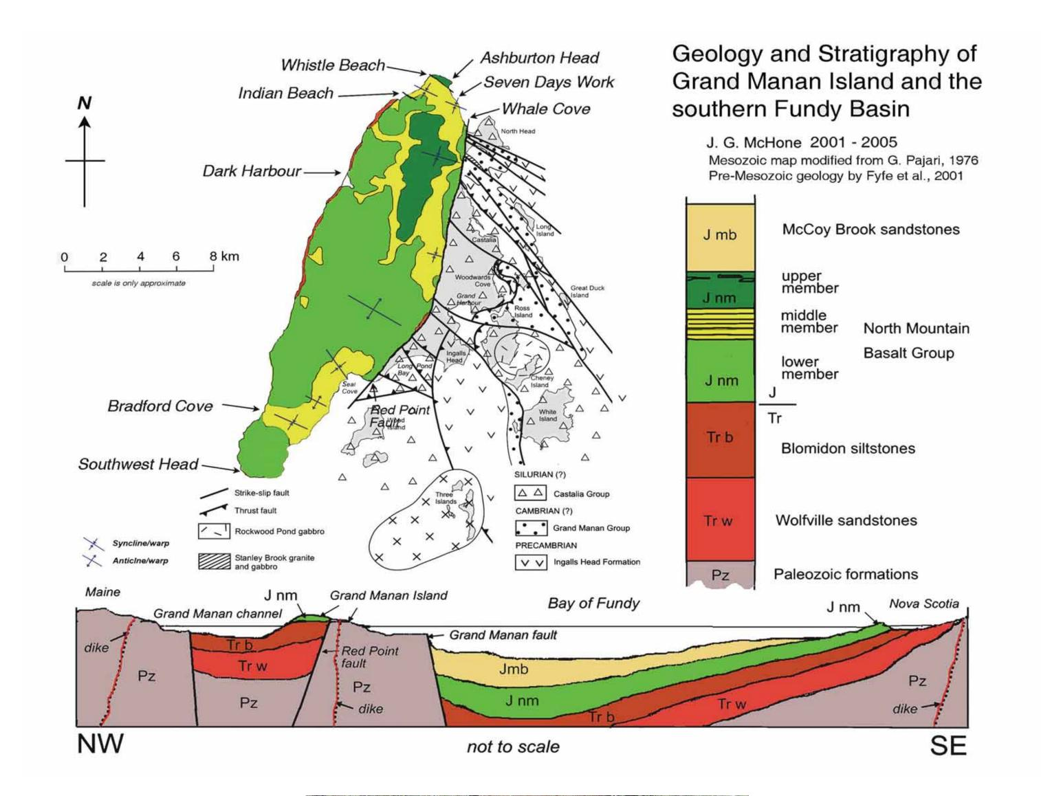
A large-displacement fault at Red Point separates the North Mountain basalts from metamorphic basement rocks that underlie the entire Fundy basin strata (right). A least several hundred meters of displacement is indicated. The fault is the eastern border of the Grand Manan sub-basin or graben, and the basement rocks to its east form a horst.
