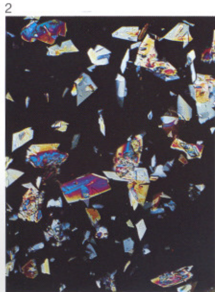
Fig. 2: Transmitted-light polarization Syllimarin (biocatalyst) with crossed polarizer and analyzer Magnification 125x Photomicrograph courtesy M. Kage, Weißenstein
