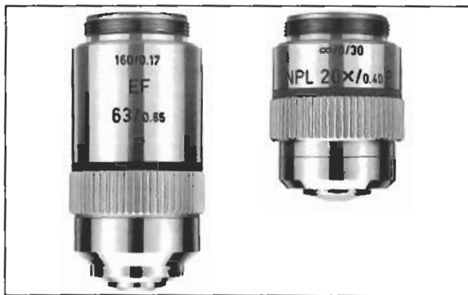
Fig. 15 Transmitted- and incident-light objective
