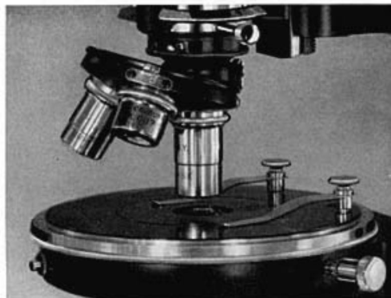
No. 455 AO triple revolving, dual-cone nosepiece on No. 42 AD.
