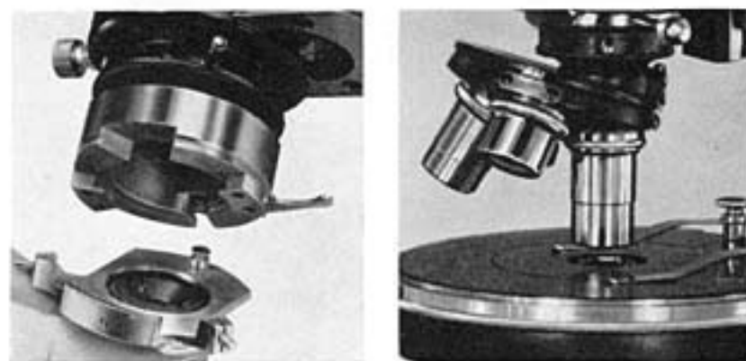
Left: Quick-change nosepiece and objective centering ring. Right: Triple-revolving nosepiece.
