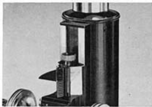
Intermediate dovetail body tube slide extends the range of the rack-and-pinion adjustment. Focusable stage is unnecessary.
